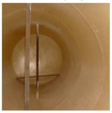
•Metallic surfaces: shot-blasting till white metal(SSPC-SP5, Svensk Sa3) and then application of **PAVIPLAST VASCHE TIX**; in case of an anti-corrosion treatment is required, or when the metal, after the sand-blasting could not be immediately coated with **PAVIPLAST VASCHE TIX**, a sand-blasting till nearly white metal is necessary (SSPC-SP10, Svensk Sa2 1/2) and then apply by brush one layer of anti-corrosion primer like FERPLAST A+B
